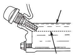
Figure 6. Engine Oil Dipstick (Oil Level)
